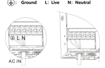
③ Correctly connect AC output wire in accordance with cable sequence and terminal position shown in the figure below. Please connect the ground wire at first, and then live wire and null wire. The ground wire is connected to the ground screw hold through Oshaped terminal.
